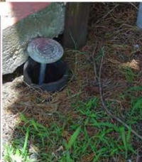
Figure 4: Estimated subsidence (in centimeters) in the New Orleans to Venice region. Photos depict relative ground subsidence of benchmarks attached to deep driven rods.
